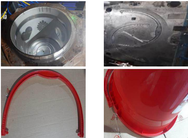
Figure 7: Injection molding and final product after modification.
