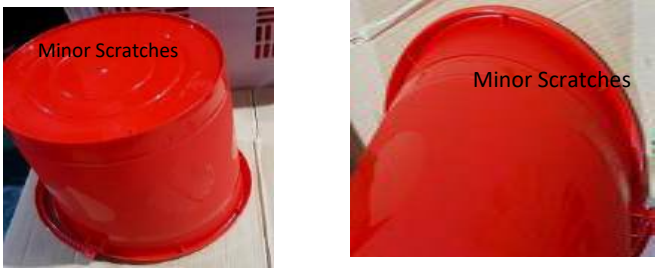
Figure 8: Condition of modified buckets after the test.
